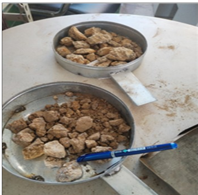
Fig. 4. Weathered sandstone encountered at deeper layers.
