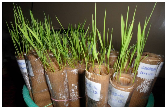
Fig. 1. Roll towel method for rice seedling germination.
