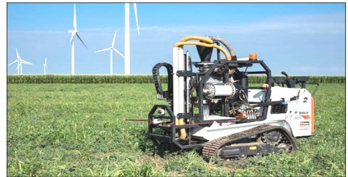
Fig. 2. Smart core robot for sampling soil.
