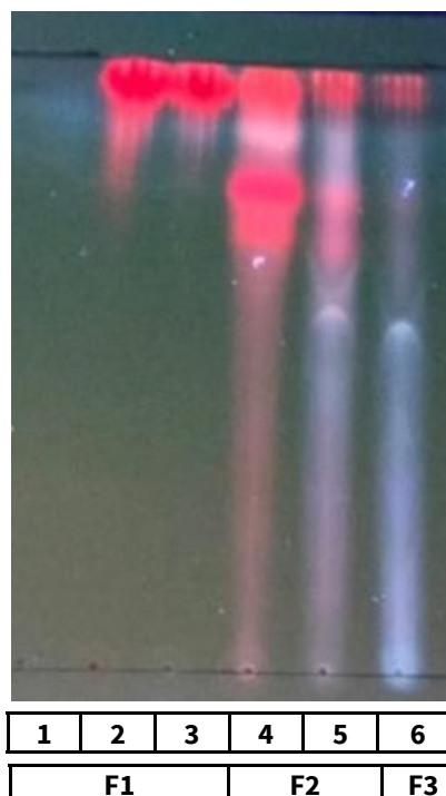
Fig. 1. Results of extract separation by thin layer chromatography (TLC). F1: fraction 1; F2: fraction 2; F3: fraction 3.
