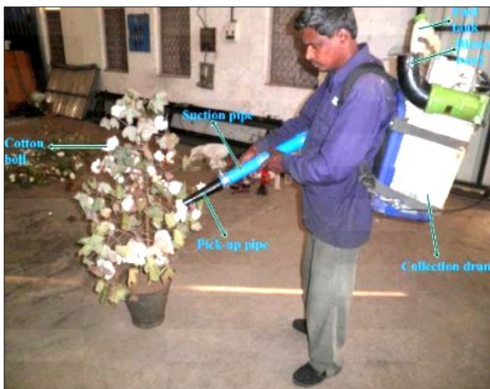
Fig. 6. Knapsack type portable engine operated cotton picker (33).
