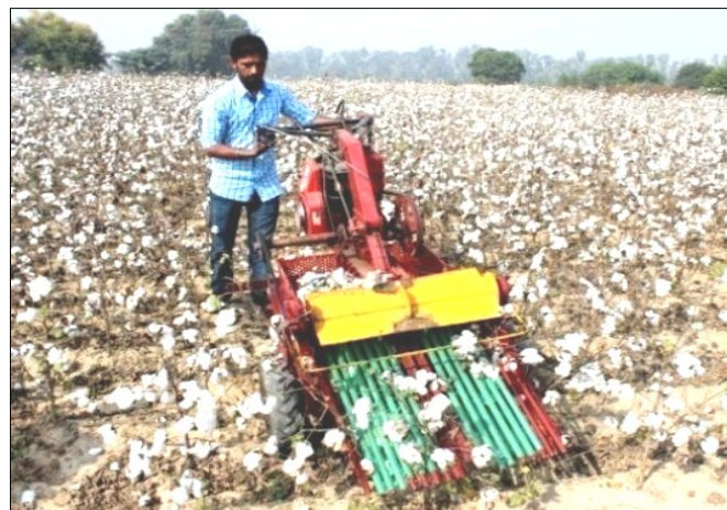
Fig. 8. Operation view of finger type cotton stripper - walk behind (55).
